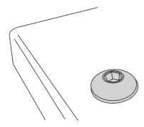
Remove the two fixing screws (3mm hexagonal socket head) and nuts that pass through the top of the rear flue grille.
